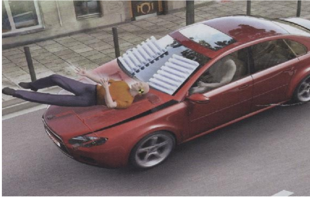
Figure 4-38: Outside Air Curtain for Pedestrian Head Protection
